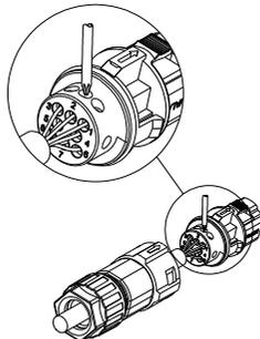
**Step 2** Push the threaded sleeve into the socket, Tighten up the cap on the terminal.
