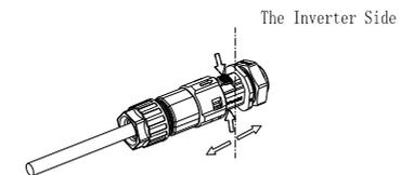
**Step 2** Insert the H type tool and pull it out from the socket.
