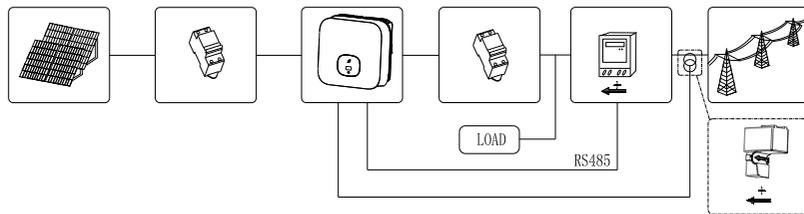
Active power control with a Radio Ripple Control Receiver(RRCR).
