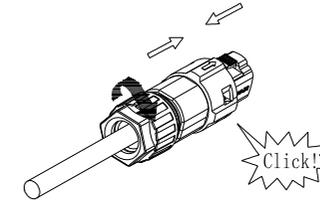
**Step 3** Push the threaded sleeve to connection terminal until both are locked tightly on the inverter.
