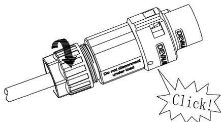
4. Finally, Push or screw the threaded sleeve to connection terminal until both are locked tightly on the inverter.
