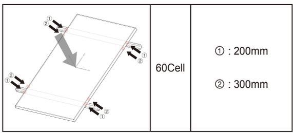
※ This mounting method is by using frame bolt holes.
