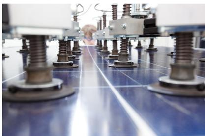
Fig. 2: Load testing at the Hanwha Q CELLS test center.
