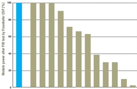
Fig. 7. In May 2012 Fraunhofer CSP tested thirteen modules from brand manufacturers – nine of the modules failed.
