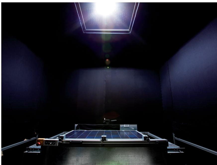
Fig. 6. Flash test: During 2012 more than 4500 solar modules were tested in the module test center. Each test usually involving power determination using the flash tester at several points in the test procedure.
